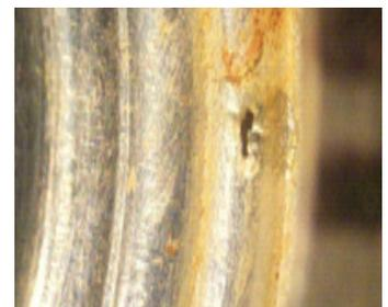
Figure 1. Galvanic corrosion in stainless steel bellows.
