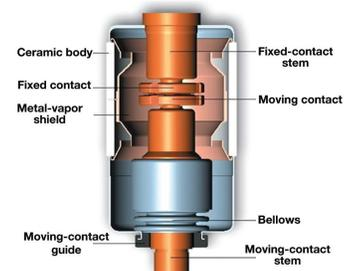
Cutaway drawing of typical vacuum interrupter.
