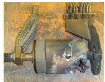
Figure 2. VI exposed to salt water then placed back into service failed catastrophically 180 days later.
