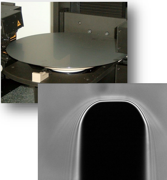
Measurement of the Edge Geometry of a Silicon Wafer
