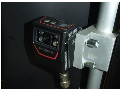
Code reader on positioning rail
