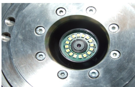
Top view of the rotary table with mounted axis camera
