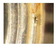
Figure 1. Galvanic corrosion in stainless steel bellows.
